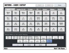
**Standard meter views** Touch a button in the lower part of the screen to view a channel, mix master, FX or matrix meter page. The page can display up to 16 meters including associated Gate, Compressor and Limiter gain reduction status indication.
